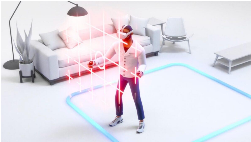
Figure 3.3 - Visual representation of the Oculus virtual boundary being crossed. Source: Meta, 2025, https://www.meta.com/nl/en/quest/safety-center/
